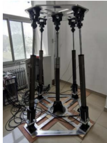
(a) Linear Stewart platform (Kharboutly et al., 2015)
